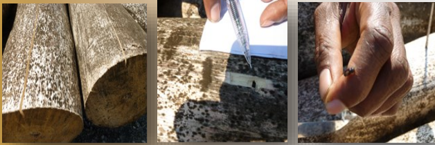
Figure 5: Blue stain and Ambrosia beetles observed outdoor air dried logs after 8 days
