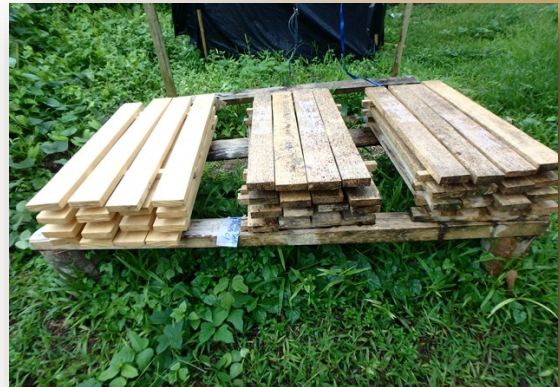
Figure 4: Blue stain observation on the outdoor experiment after one month
