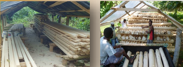
Figure 3: Storing of poles and timber at operation site
